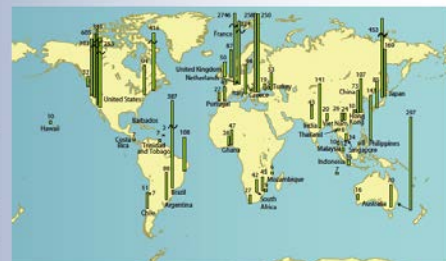
Figure 5: Concentration of PCBs in beached plastic resin pellets, in nanograms per gram of pellet. Samples of polystyrene pellets have been collected at 50 beaches in 29 countries and analyzed for concentrations of organochlorine compounds. PCB concentrations were highest in pellets collected in the United States, Western Europe and Japan. They were lowest in those collected in tropical Asia and Africa. This spatial pattern reflects regional differences in the use of PCBs. Source: Ogata et al. (2009) with additional data provided by International Pellet Watch in 2010
